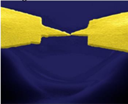
Single Molecule Diode
